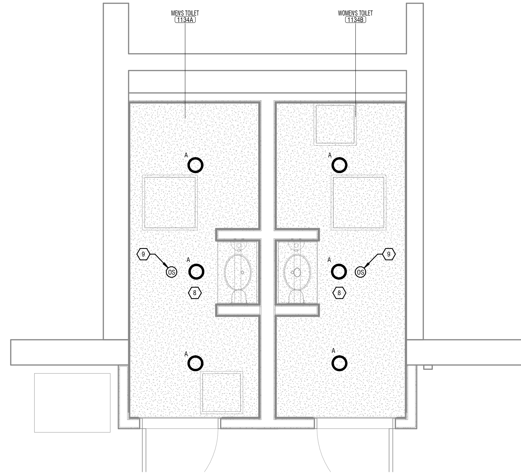
4 ROOMS 1134 A & B - LIGHTING INSTALLATION E-101 1/2" = 1'-0"
